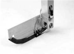
Fig. 3. In practice, we obtained the best results with a foot radius of 25 [cm], a foot length of 13 [cm], and a forward displacement of 6 [cm]. The foot switch allows the controller to adapt to the actual step time by registering the exact instant of heel strike
